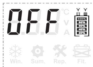
Automatically Shut Down In 2 Hours After Fully Charged
