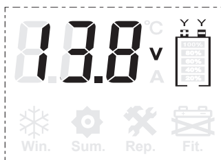
Icon Blinks When Connected Improperly
