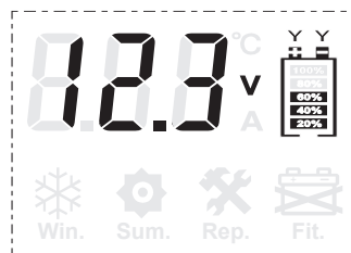
Normal Charging When Current, Voltage And Temperature Display In Rotation, And Power Level Blinks Successively
